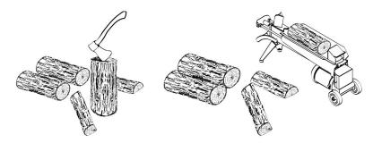
Wood should be split to a range of sizes, from about 3" to 6" (75 mm to 150 mm) in cross section. Having a range of sizes makes starting and rekindling fire much easier.
