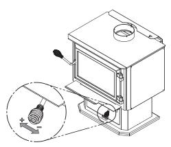
On the other hand, too much air can make the fire uncontrollable, creating very high temperatures in the unit as well as in the chimney and seriously damaging them. A reddish glow on the unit and on the chimney components indicates overheating. Excessive temperatures can cause a chimney fire.
