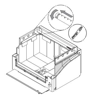
Note that secondary air tubes **(B)** can be replaced without removing the baffle board **(A)** and that all tubes are identical.
