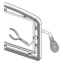
Removing the retaining pin
