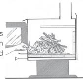
Then add two or three small pieces of firewood. Open the air intake control completely and ignite the newspaper. Leave the door slightly ajar. Once the fire has ignited, the door can be closed with the air control still fully open. When the kindling is almost completely burned, standard firewood pieces can be added.
