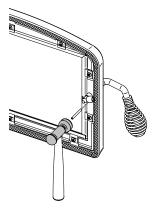
Reinstalling the retaining pin
